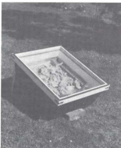
Solar Wax Melter: an ideal way for the hobbyist to deal with wax scrapings and cappings wax.
